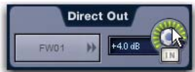
Adjusting Direct Output level from the Patchbay
