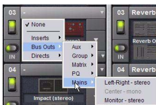
Assigning monitor output to a bus-fed plug-in
