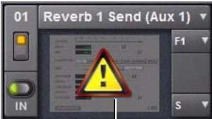
Unavailable plug-in Indication of an unavailable plug-in
