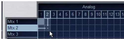
Assigning an output in the Patchbay Outputs page
