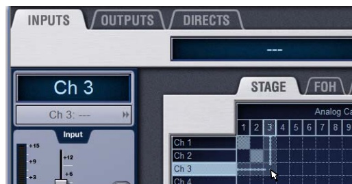
Assigning input sources in the Patchbay Inputs page
