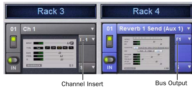
A mono plug-in inserted on a channel (at left) and a stereo plug-in assigned as a bus processor (at right)
