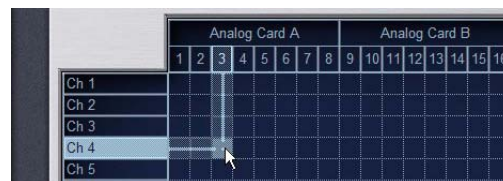
Routing a hardware input to an Input Channel
