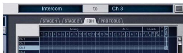
Routing Intercom input in the Patchbay
