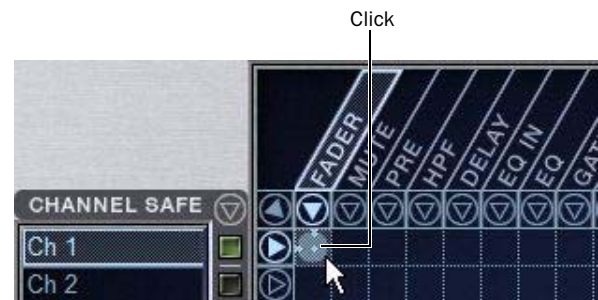
Enabling recall safe for channel 1 fader
