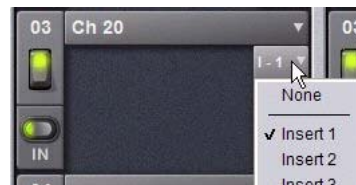
Channel Insert selector for a plug-in rack
