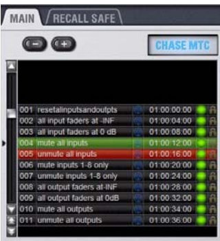
Snapshot list with Center Last Recalled Snapshot enabled
