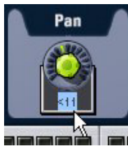
Adjusting a parameter value by dragging over its text box
