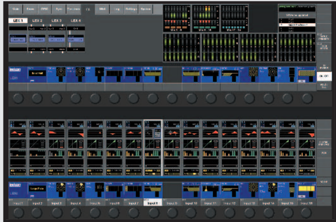
LEXICON FX Simple touch selection of reverb type accompanies full parameter control on the rotary encoders. FX may be patched into inputs, channel inserts or aux busses.
