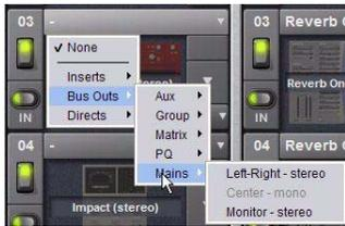
Assigning monitor output to a bus-fed plug-in
