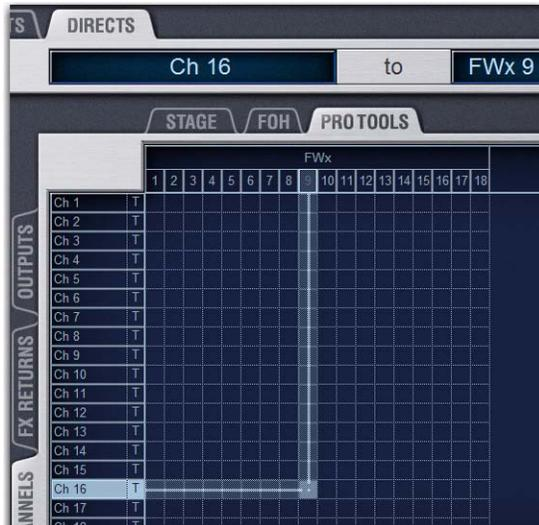
Routing a Direct Output to an FWx channel
