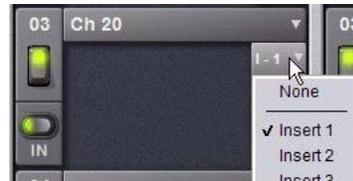
Channel Insert selector for a plug-in rack
