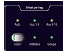
*Bus output LEDs and Select switch*
