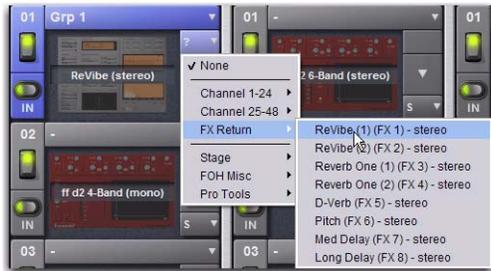
Assigning plug-in output to an FX Return
