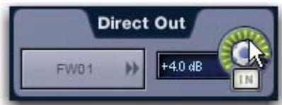
Adjusting Direct Output level from the Patchbay
