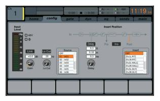
The *config* tab of input channels 1-32 contains the following parameters that can be adjusted using the six push encoders:
