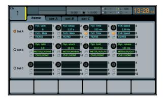
The **ASSIGN** screen's *home* tab provides a visual overview of the 12 assigned controls for all three sets at the same time.
