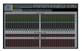
The **METERS** screen displays different groups of level meters for various signal paths on the console, and is useful for quickly ascertaining if any channels need level adjustment. Since there are no parameters to adjust for the metering displays, none of the metering screens (with the exception of the rta tab; see below) contain any 'bottom-of-screen' controls that would normally by adjusted by the six push encoders.
