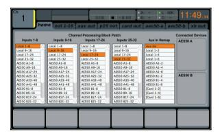
The **ROUTING** screen is where all signal patching is done, allowing you to route internal signal paths to and from the physical input/output connectors located on the M32's rear panel.
