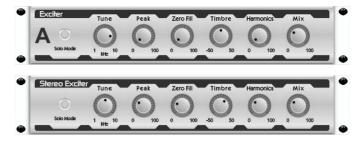
Exciters increase presence and intelligibility in live sound applications, and are indispensable for adding clarity, air and harmonic overtones in the recording studio. This effect is particularly useful for filling out the sound in difficult rooms, and for producing a more natural live or recorded sound. *Inspired by the famous Aphex Aural Exciter.*
