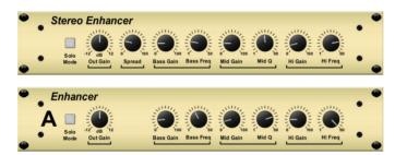
The M32's Enhancers are so called 'Psycho EQs'. They can enhance the signal spectrum in bass, midrange and high frequencies, but they differ from traditional EQs. When you need to generate maximum punch, clarity and detail, without turning up the overall volume, our enhancers are the solution. *Inspired by the SPL Vitalizer*.
