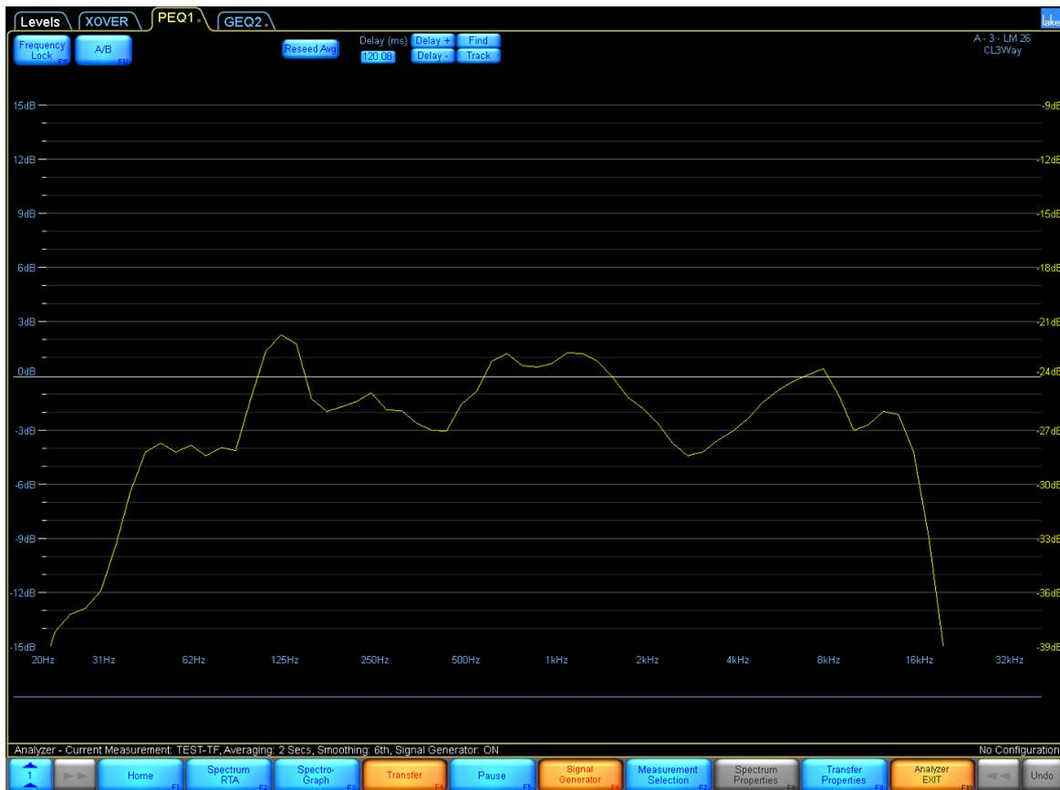
**Figure 17-12: Transfer function measurement mode**
