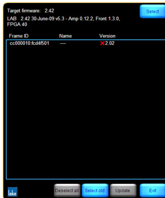
**Figure 25-3: PLM Firmware Utility Main Screen**
