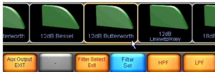
**Figure 7-22: Selecting a new filter slope for HPF or LPF**
