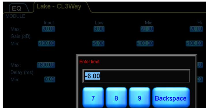
**Figure 18-8: Restricting the Minimum Gain Value for Output 1**
