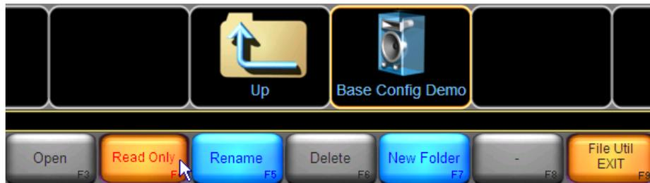
**Figure 18-5: Setting a Base Config File to Read Only**
