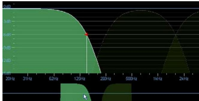
**Figure 4-46: Splitting and moving the low channel HPF**
